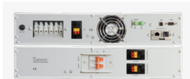
RT Industrie 3 kVA rear panel with external battery pack (bottom) and hardwired input and output
