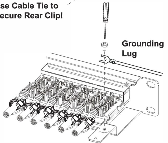
Tightening the ground lug with screw.
