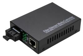
Each Media Converter provides a 10/100/1000BaseT/TX auto-negotiating RJ-45 twisted-pair connector port featuring store-and-forward switching architecture. The Built-in switch does the network segmentation to provide the maximum fiber distance. Auto-MDIX capability on the twisted-pair port allows convenient connection.
