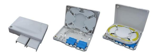
TH-002 is a 4 Fibre Compact Termination Box, designed for use in residential and business applications for the termination of up to four fibres. The wall box enables the installation of either a single Blown Tube cable using up to a 4 fibre blown unit or two 2 fibre ruggedised cables to be spliced to four SC pigtails (PC or APC), which connect to adapters at the base of the unit.
