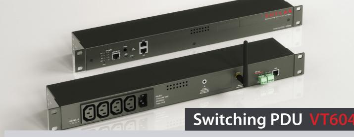
Device is used for load management and allows to switch on/off or reboot up to 4 outlets. It has built-in temperature sensor, two ports for analog sensors, two dry contacts, two12V outputs for devices (for example, alarm beacons), USB port for camera, a slot for GSM modem and allows to connect up to 4 IP cameras.
