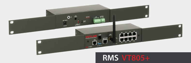
The unit is used for environmental control in different facilities. Can connect up to 30 sensors, 4 dry contacts, two 12V alarm beacons, GSM modem, USB camera, four IP cameras, SD card for logs, 1-Wire board with 1-Wire sensors. Has a built-in web interface & supports protocols like HTTP, HTTPS, SNMP v1, 2c, 3, SMTP, Radius, Syslog and other.
